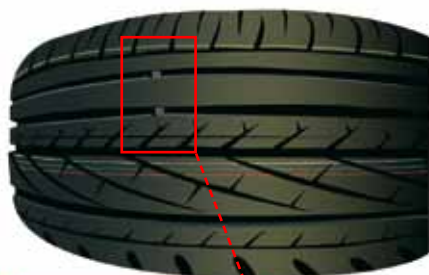
TWI (Tread Wear Indicator) – with the limit value of 1.6mm.
